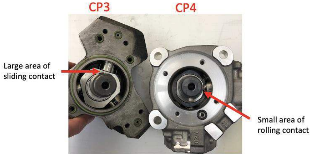
Figure 3: Comparison of CP3 and CP4 Pumps
