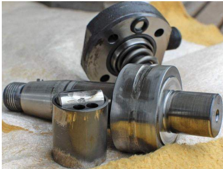
Figure 6: Wear on the Cam and Roller
